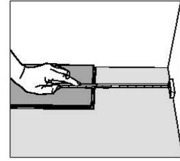
④ At the end of the first row, leave an expansion gap of  $\frac{1}{4}$ " to the wall and measure the length of the last plank to fit.
