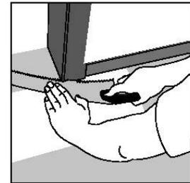
⑫ Door molding and skirting: lay a board (with the decorative side down) next to the door molding and as shown in the figure. Then slide the floorboard under molding.
