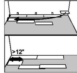
⑥ Start the second row with the leftover cut part of the last plank of the previous row. This small plank should measure at least 12". Otherwise, use another plank that should be cut in two. The end joints of each adjoining row should not be closer than 8" to each other.
