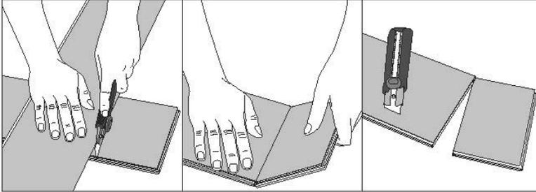
⑤ To cut the plank, use a simple utility knife and ruler, and with the top side facing up, cut heavily and several times on the same axis. The knife will not go through the surface but make a deep cut. You can then lift one half of the plank using your other hand to hold down the second placing it very close to the cut. The plank will split naturally.
