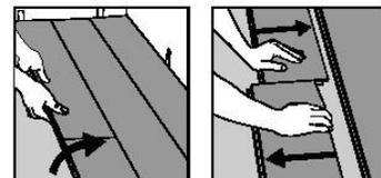
Separate the whole row by lifting it up delicately at an angle. To separate the planks, leave them flat on the ground and slide them apart. If planks do not separate easy, you can slightly lift up the planks (5") when sliding them apart.
