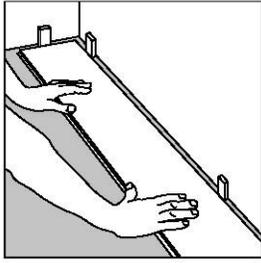
① After thoroughly cleaning the subfloor, you should begin laying in the left-hand corner. Place the floorboard  $\frac{1}{4}$ " from the left wall. Use spacers between the wall and the floorboard.
