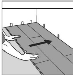
⑨ After 2-3 rows. Adjust the distance to the front wall by leaving an expansion gap of  $\frac{1}{4}$ ". Always ensure that the end joints are staggered at least 8", both when in the same row as when from one row to the next one.
