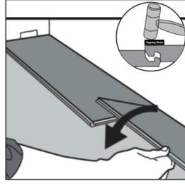
② Second Plank, first row; lower the plank until it is resting in line with the adjacent plank. Firmly strike the surface of the locking mechanism with a Soft Faced Hammer and a tapping block until the planks are locked together at the same height. Make sure both planks are perfectly aligned.
