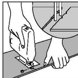
⑪ Holes for pipes: measure the diameter of the pipe and drill a hole that is  $\frac{1}{8}$ " larger. Saw off a piece as shown in the figure and lay the board in place on the floor. Then lay the sawed-off piece in place.
